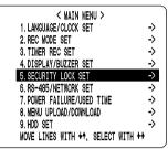
You can set passwords that restrict use of the digital video recorder to administrators and designated users, preventing unauthorized operation. When the security lock is set, a buzzer sounds when an unauthorized user presses any of the digital video recorder's operation buttons. Be sure to make a note of the set passwords.
